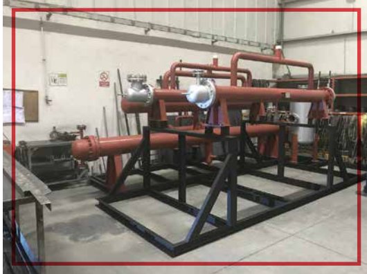
KGS Proses CO 2 -NH 3 heat exchangers & Pressure vessels
